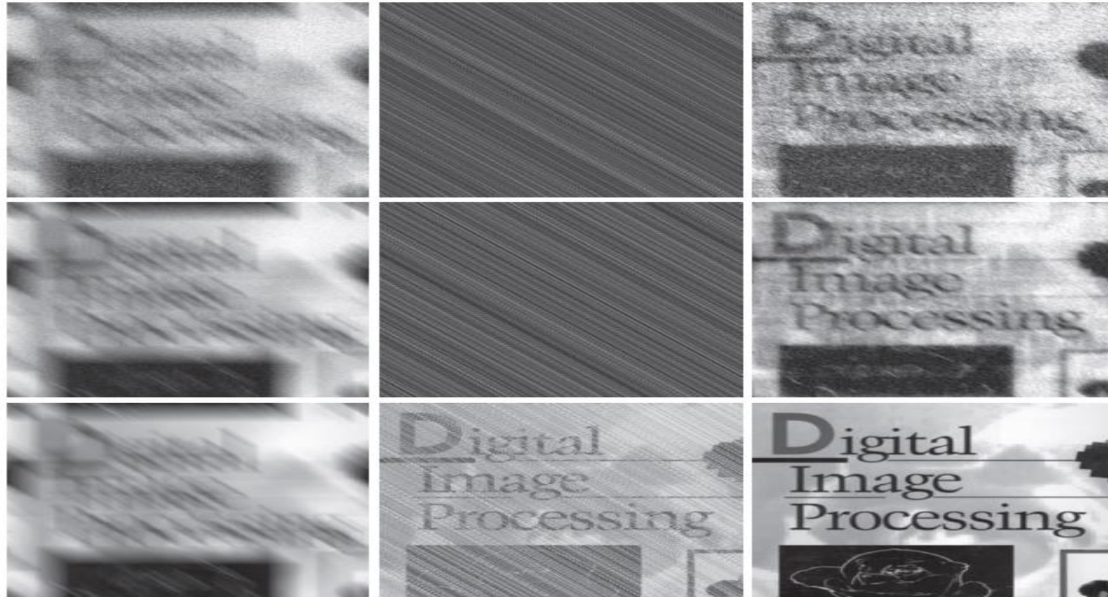
FIGURE 5.29 (a) 8-bit image corrupted by motion blur and additive noise. (b) Result of inverse filtering. (c) Result of Wiener filtering. (d)–(f) Same sequence, but with noise variance one order of magnitude less. (g)–(i) Same sequence, but noise variance reduced by five orders of magnitude from (a). Note in (h) how the deblurred image is quite visible through a “curtain” of noise.
